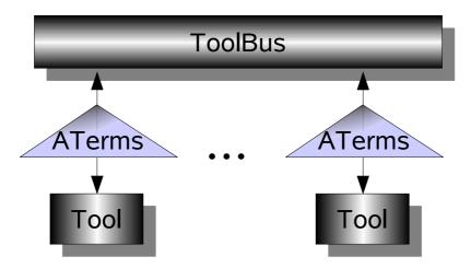
Figure 4: The TOOLBUS coordination architecture.
