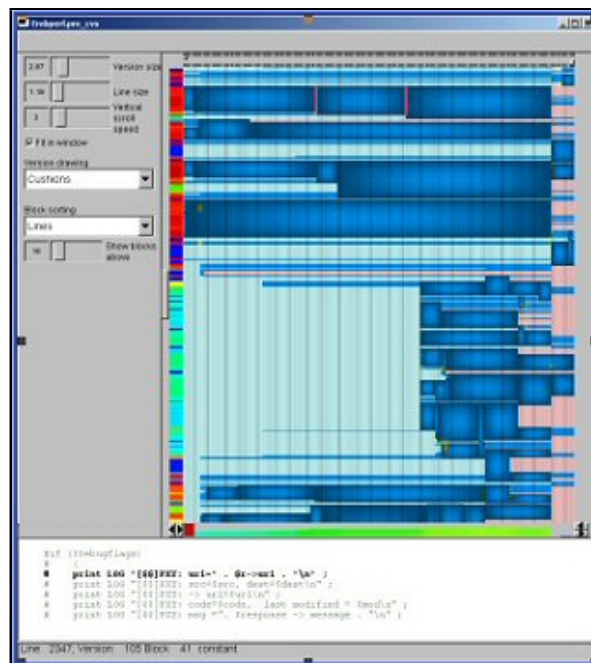
Figure 3.2: The CVSScan visualization displays the evolution of a single source code file. The visualization shows every different version of the code and can even trace where the code originated and how much of it is still left.
