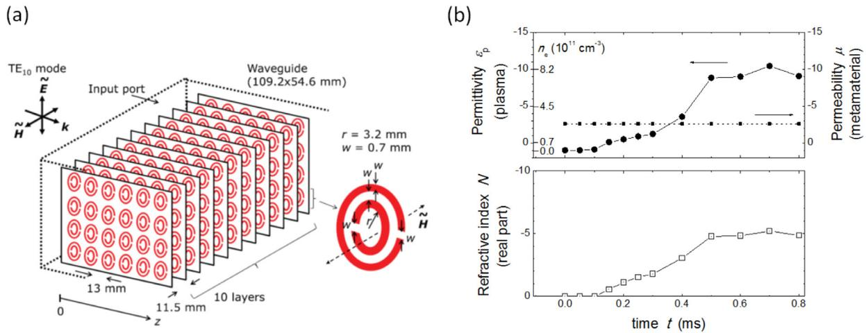
**Figure 4.** (a) Schematic of magnetically-active metamaterial that is inserted into an argon-filled waveguide section in which plasma is formed by pulsed excitation. (b) Time-variation in the measured dielectric constant and corresponding refractive index within the metamaterial-filled section. Note transition to negative values due to plasma density evolution to above cut-off values.
