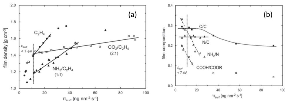
**Figure 9.** Comparison of film density (a) and functional group density (b) for plasma-based deposition of plasma-polymer films versus momentum transfer to the surface during deposition. Reprinted from [53], with the permission of AIP Publishing.
