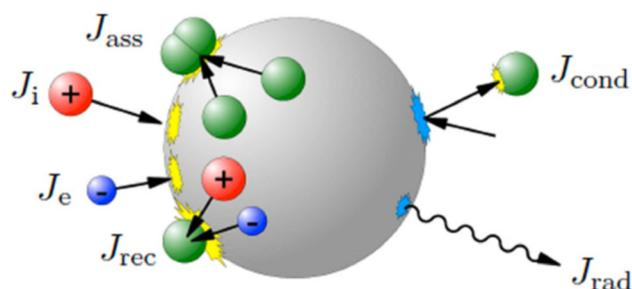
**Figure 13.** Schematic of the energy exchanges between nanoparticles and the surrounding plasma. Nanoparticles receive energy through energetic surface reactions, such as electron and ion bombardment, recombination, and association reactions. They lose energy through conduction to the neutral gas and radiation. Reproduced from [74]. © IOP Publishing Ltd. All rights reserved.
