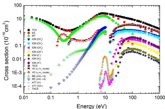
**Figure 34.** Summary of recommended cross section for electron collisions with methane: TCS—total scattering, ES—elastic scattering, MT—momentum transfer, ION—partial ionization, TICS—total ionization, VE—vibrational excitation, RE—rotational excitation, ATT—dissociative attachment, TACS—total dissociative attachment. Reprinted from [177], with the permission of AIP Publishing.
