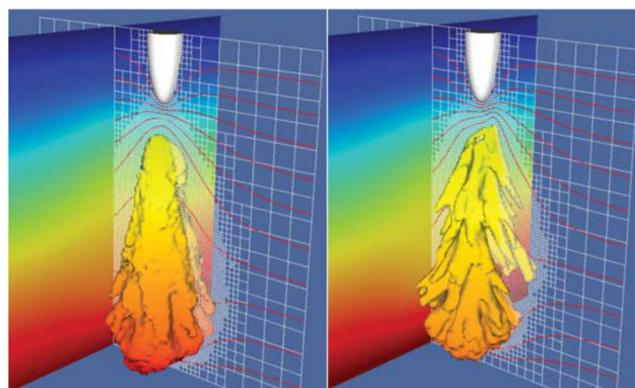
**Figure 32.** Particle in cell simulation of breakdown in 100 Torr of argon for point-to plane potential of (left) 3.25 kV and (right) 5 kV using AMR techniques. Isosurfaces of electron density ( $10^{16} \text{ m}^{-3}$  and  $5 \times 10^{16} \text{ m}^{-3}$ ), adapted grids, and equipotential lines are shown. Reproduced from [164]. © IOP Publishing Ltd. CC BY 3.0.
