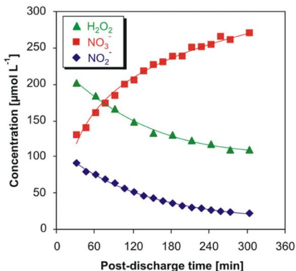
**Figure 27.** Post-discharge evolution of H<sub>2</sub>O<sub>2</sub>, NO<sub>2</sub><sup>-</sup> and NO<sub>3</sub><sup>-</sup> in aqueous solution (pH 3.3) after treatment by the air discharge plasma. Reproduced from [140]. © IOP Publishing Ltd. All rights reserved.
