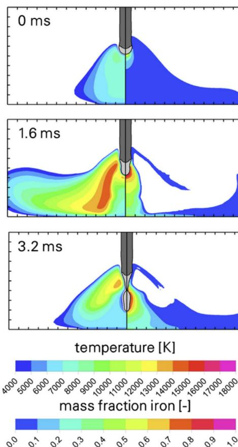
**Figure 24.** Calculated distributions of arc temperature (left) and iron vapour mass fraction (right) at different times in pulsed metal–inert-gas welding of iron. The arc current at the successive times is 50, 420 and 150 A, respectively. The changes in location of the iron vapour production as the arc current changes lead to changes in the distribution of current density and temperature in the arc. Springer [125] © International Institute of Welding 2016, with permission of Springer.
