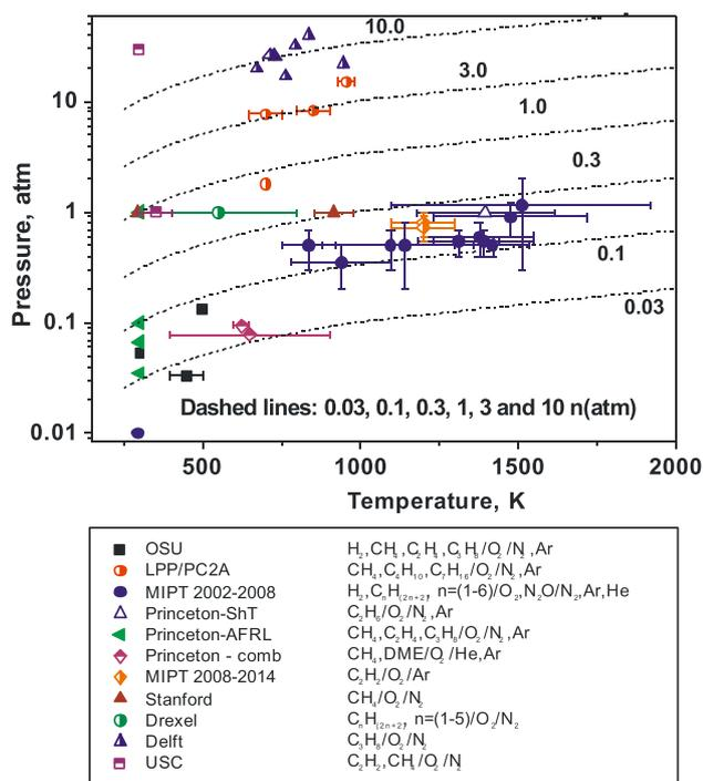
**Figure 21.**  $P$ – $T$  diagram [113] of results available in the literature from experiments on combustion initiated or assisted by nanosecond discharges. Dashed lines are the isolines of the gas density, normalized with respect to the atmospheric gas density  $n_{atm}$  for normal conditions. Reproduced from [113]. © IOP Publishing Ltd. All rights reserved.
