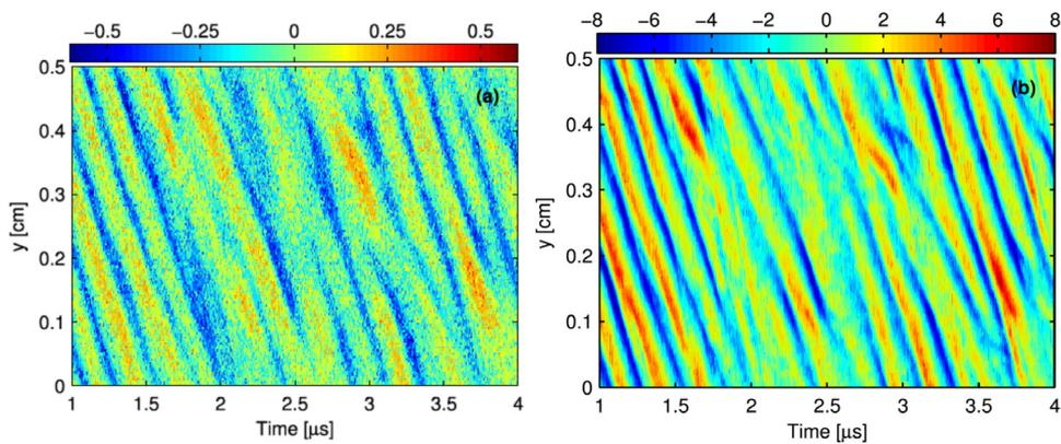
**Figure 31.** Contour plots of (a) electron density and (b) electric field showing MHz scale frequency fluctuations in a particle-in-cell simulation of a Hall thruster. Reprinted from [156], with the permission of AIP Publishing.
