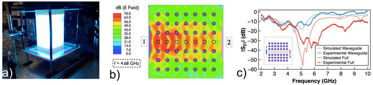
**Figure 3.** (a) Photograph of a plasma photonic crystal array comprised of  $7 \times 7$  high current density discharge tubes. (b) Simulated waveguide performance when a row of the discharges is turned off and an antenna is placed at location 1, to transmit an EM wave to location 2. (c) Comparison of measured and simulated transmission ( $S_{21}$ ) spectra for the configuration in (b).
