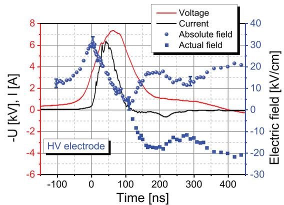
**Figure 8.** Electric field in quasi-2D ns pulse discharge ‘curtain’ plasma in ambient air, measured by ps 4-wave mixing  $\sim 100 \mu\text{m}$  from the high-voltage electrode. The discharge is sustained between a steel razor blade and grounded copper foil covered by a quartz plate with a thickness of  $120 \mu\text{m}$ . The discharge gap is  $600 \mu\text{m}$ . Reproduced from [45]. © IOP Publishing Ltd. All rights reserved.
