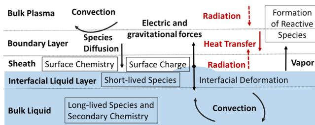
**Figure 5.** Schematic representation of the key plasma–liquid interactions. The boundary layer reflects the gradients in temperature, species densities and gas flow velocities. The sheath is present for ionizing plasmas when the liquid surface is charged.
