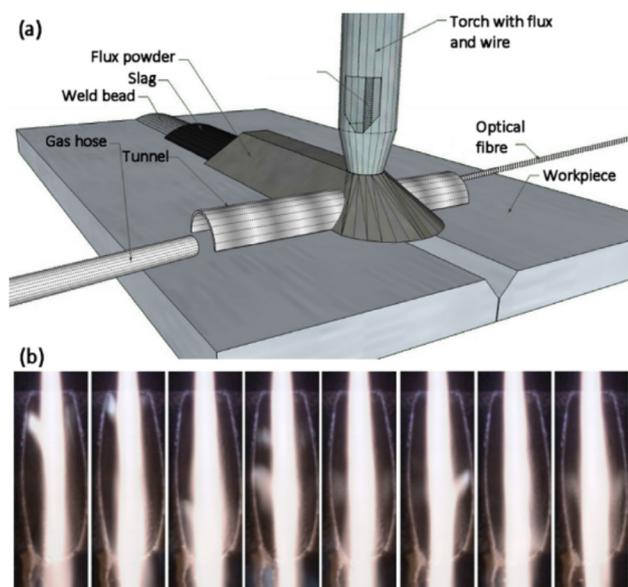
**Figure 25.** Innovative methods for imaging ‘hidden’ regions: (a) placement of a tunnel through a submerged arc weld. [127] *Welding Journal*, (August 2015) © American Welding Society. (b) High-speed images of piercing of the edge of a 20 mm steel plate by the plasma cutting arc with constant time steps of 0.033 ms, showing the arc root attachment. Springer [128] © Springer Science + Business Media, LLC 2011, with permission of Springer.
