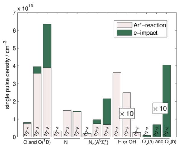
**Figure 16.** Results from a model of a shielded Ar kinpen device at atmospheric pressure with predictions of RONS densities generated by a single guided streamer at dry synthetic air mole fractions  $10^{-4}$ ,  $10^{-3}$  and  $10^{-2}$ . Contributions from direct electron impact reactions and reactions involving excited argon species are distinguished: note the importance of Ar metastables as reactive precursors in this study. Reproduced from [88]. © IOP Publishing Ltd. All rights reserved.
