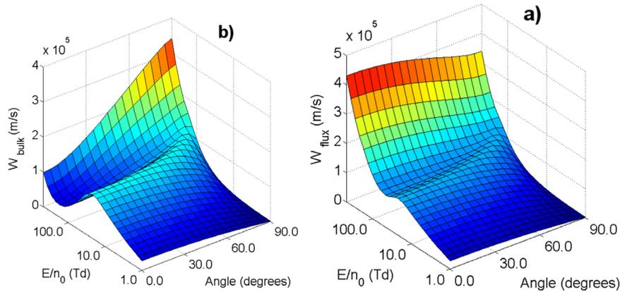
**Figure 7.** Multi-term solutions of the Boltzmann equation for drift velocities (a) bulk and (b) flux for positrons in  $\text{CF}_4$  in combined electric and magnetic fields for  $B/n_0 = 1000$  Hx, (in units Huxley,  $1 \text{ Hx} = 10^{-27} \text{ Tm}^3$ ,  $n_0$  is the gas number density) as a function of  $E/n_0$  (in units Townsend  $1 \text{ Td} = 10^{-21} \text{ Vm}^2$ ) and the angle between the two fields.
