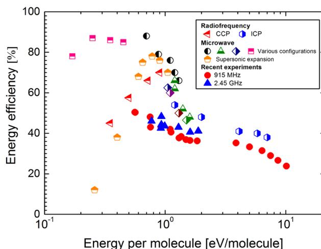
**Figure 20.** The energy efficiency of CO<sub>2</sub> dissociation for various plasma reactors (CCP capacitively coupled plasma, ICP inductively coupled plasma and microwave plasmas (flow and supersonic expansion)). Data taken from [106, 107] with recent results from the DIFFER institute using flowing microwave reactors.
