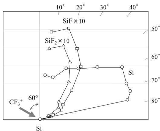
**Figure 10.** Angular distributions of desorbed species when a single crystal Si (100) surface is exposed to a 500 eV  $\text{CF}_3^+$  beam at an incident angle of  $60^\circ$ . The radius of the polar graph (i.e. the distance between the origin and a point on the curve) is proportional to the flux of desorbed species. Reproduced from [56]. © IOP Publishing Ltd. All rights reserved.
