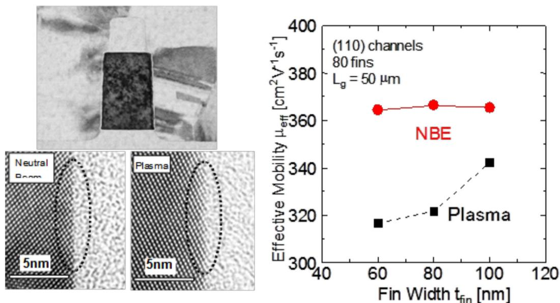
**Figure 11.** Dependence of Si channel electron mobility on fin width. Neutral beam and plasma was used for etching. Higher mobility Si channel was obtained using neutral beam etching. Reproduced with permission from [62].
