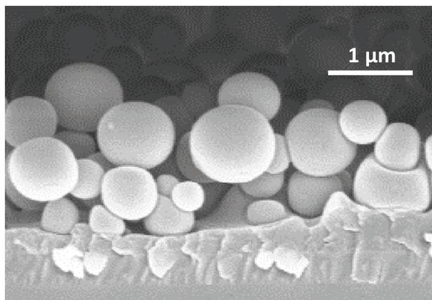
**Figure 12.** Core-shell nanocapsules produced in an aerosol-assisted AP PE-CVD process. The shell is made of a hydrocarbon membrane originated from the ethylene feed in the discharge. The core contains a droplet of a biomolecule solution.
