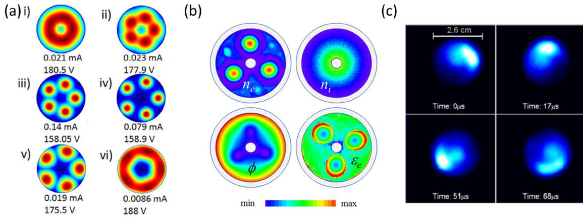
**Figure 30.** (a) Cathode spots calculated from a theoretical model. Reproduced from [154]. © IOP Publishing Ltd. All rights reserved. (b) Electron density, ion density, potential and electron energy calculated from a particle-in-cell simulation of a magnetron. Reproduced from [152] CC BY 3.0. (c) Visible light emission from a rotating spoke in a Hall thruster experiment. Reprinted from [155], with the permission of AIP Publishing.
