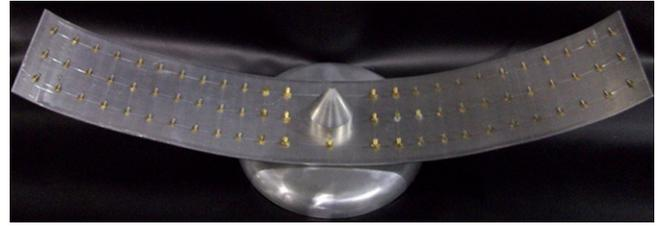
**Figure 6.** Our alternative grounded electrode of 55 by 10 cm<sup>2</sup> with 75 sharp points to generate upward negative streamers.
