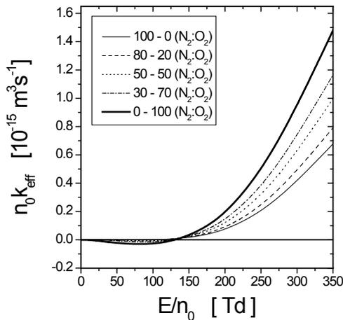
**Fig. 1.** Variation of the effective ionization coefficient with  $E/n_0$  for various N<sub>2</sub>-O<sub>2</sub> mixtures.
