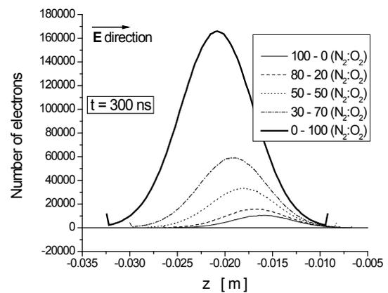
**Fig. 2.** The spatial distribution of the electron swarm for various N<sub>2</sub>-O<sub>2</sub> mixtures.
