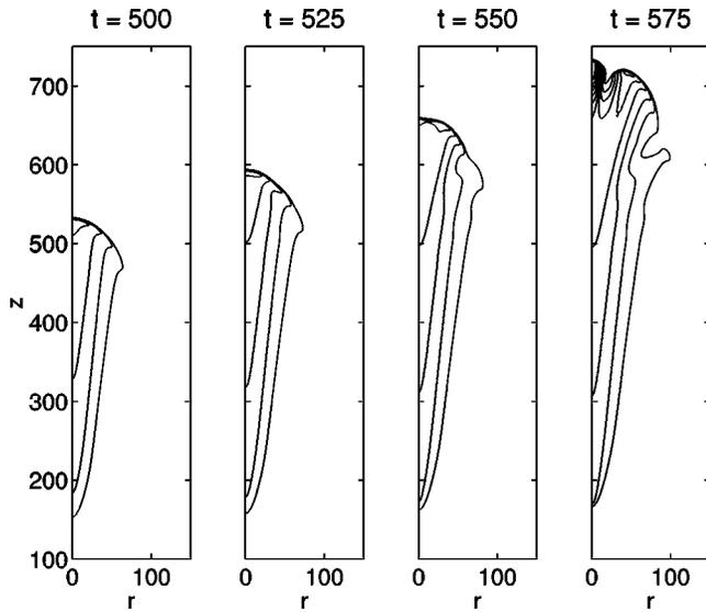
FIG. 1. Evolution of an anode directed streamer in a strong homogeneous background field. The planar cathode is located at  $z = 0$  and the planar anode at  $z = 2000$ . The radial coordinate extends from the origin up to  $r = 2000$  to assure homogeneous field conditions. Shown is  $100 \leq z \leq 750$  and  $0 \leq r \leq 150$  with equal axis scaling. The thin lines denote levels of equal electron density  $\sigma$  with increments of 0.15. All plotted quantities are dimensionless.
