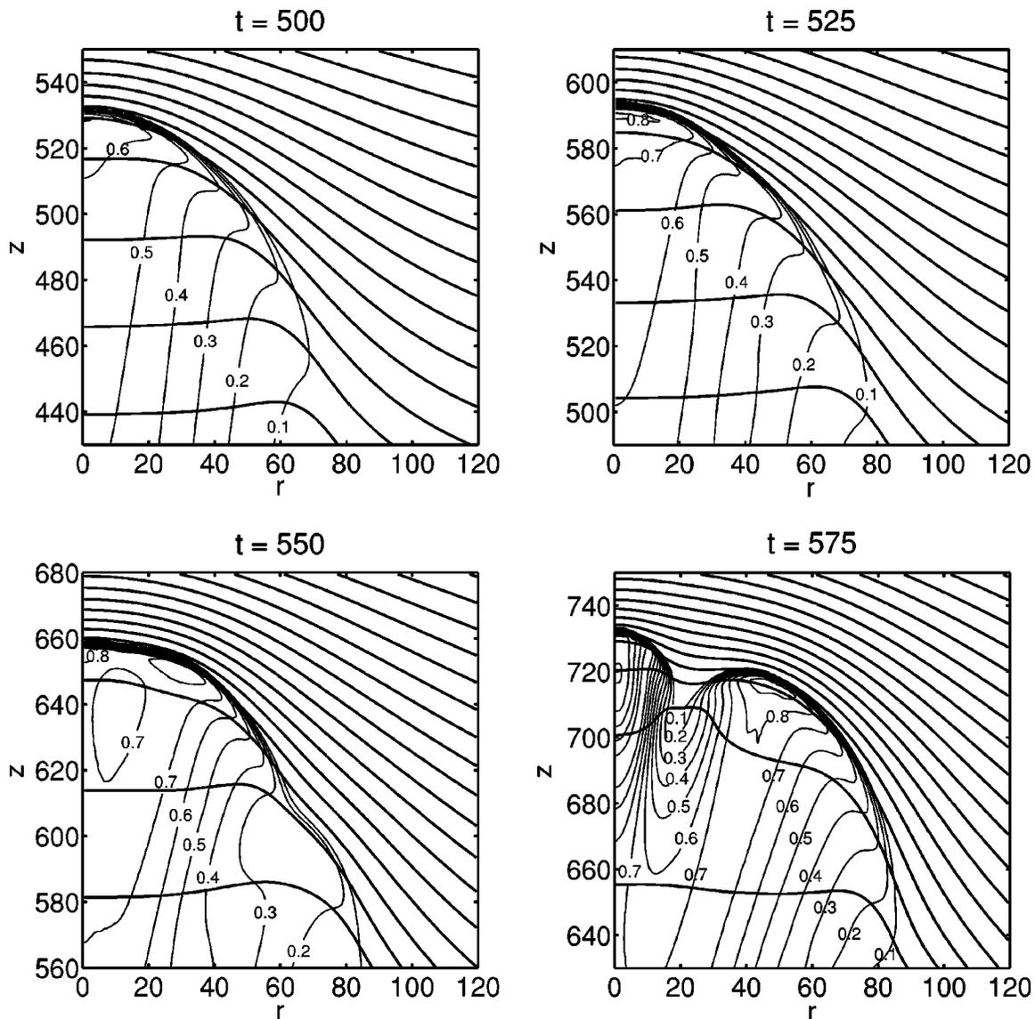
FIG. 3. Enlargement of the evolution of the streamer tip showing electron density  $\sigma$  with increments of 0.1 as thin lines and electric potential  $\Phi$  with increments of 5 as thick lines. At the last time step  $t = 575$ , the maximal electron density in the core of the finger on the axis is 1.5. All figures have equal aspect ratio and equal axis scaling.
