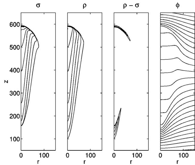
FIG. 2. The streamer at time  $t = 525$ . The figures show contour plots with equal aspect ratio for the electron density  $\sigma$ , ion density  $\rho$ , space charge density  $\rho - \sigma$ , and electric potential  $\Phi$ . The level lines for the densities  $\sigma$  and  $\rho$  are multiples of 0.1, for the space charge density  $\rho - \sigma$  of 0.05, and the increment between different levels of the potential is 10.
