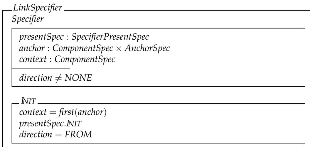
By default, the specifier is initialized to represent the most simple case, i.e. where the context component equals the component containing the anchor.
