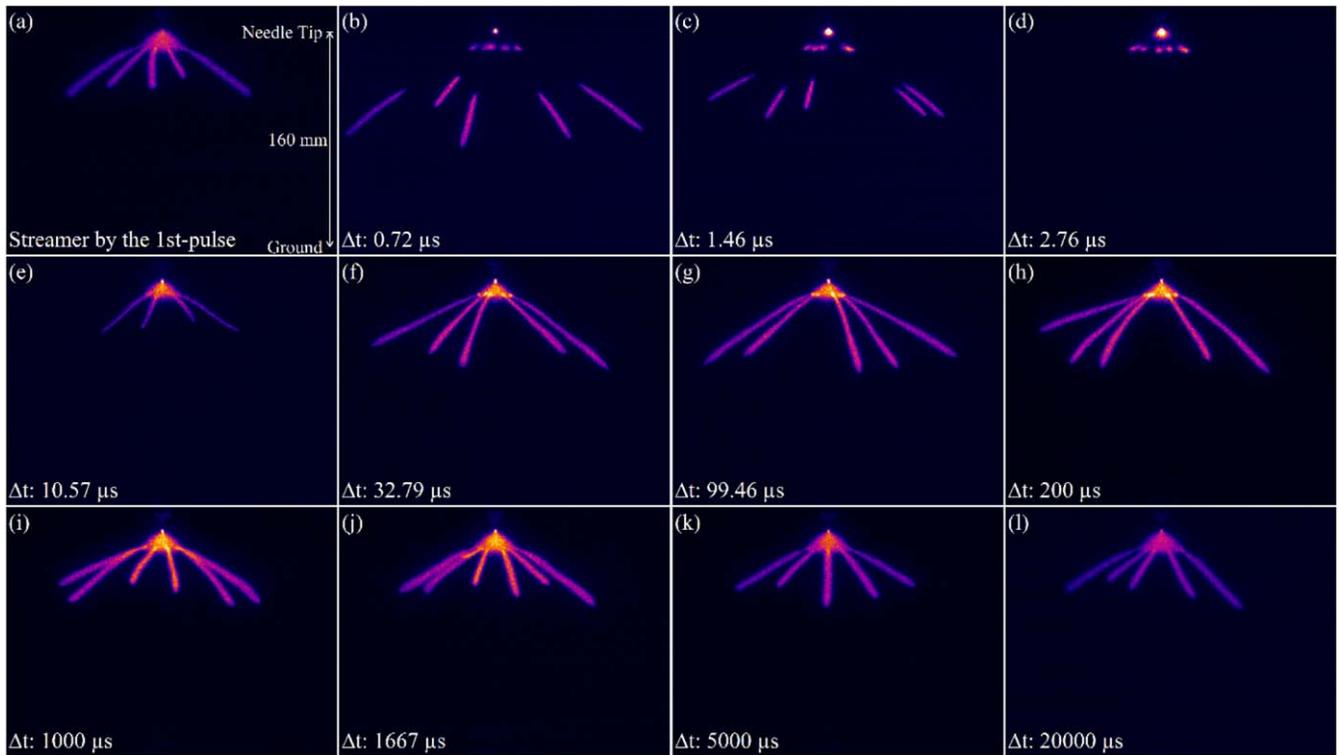
**Figure 4.** First pulse streamer (panel (a)) and second pulse streamers (panels (b)–(l)) in 66.7 mbar artificial air with varying pulse-to-pulse delay ( $\Delta t$ ) with 6.6 kV amplitude and 500 ns pulse width.
