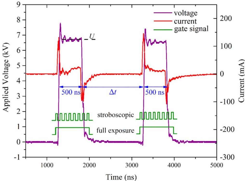
**Figure 1.** Typical double-pulse voltage, current and two kinds of imaging techniques (full exposure and stroboscopic imaging). The shown example has 6.6 kV voltage, pulse lengths of 500 ns and a pulse-to-pulse delay  $\Delta t = 1.4 \mu\text{s}$  in 100 mbar pure nitrogen.
