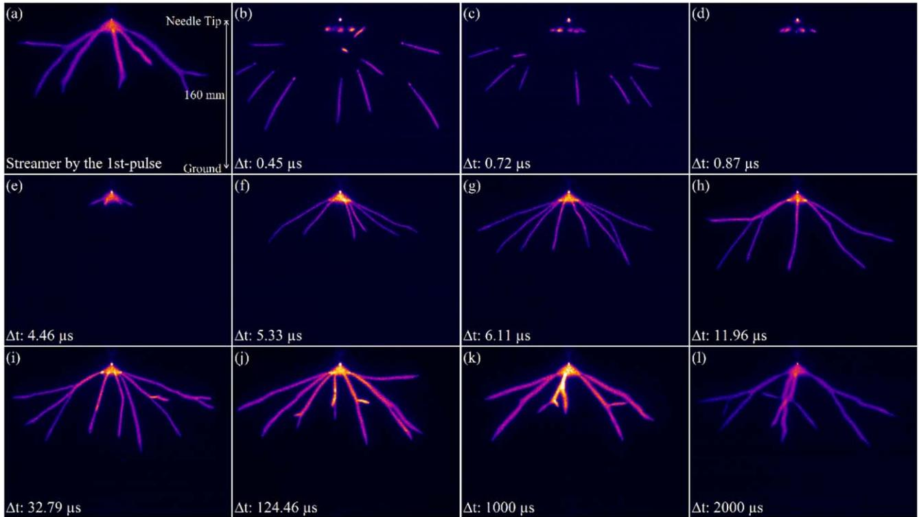
**Figure 5.** The same as figure 4, now in 100 mbar artificial air with 8.5 kV voltage amplitude.
