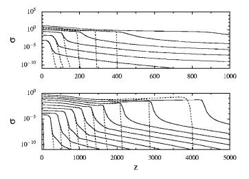
FIG. 3. Evolution of the logarithmic electron density on the streamer axis at pressure  $p \leq 60$  Torr (solid lines) and without photoionization (dashed lines) in the high field (above), corresponding to columns 2 and 4 in Fig. 2 and low field (below), which corresponds to the upper and lower plots in the left column of Fig. 2.
