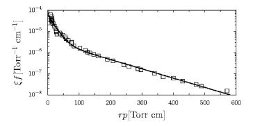
FIG. 1. Function  $\xi f$  of the photoionizing radiation in the range of 980 -1025 Å in air, taken from Ref. 15 (squares) and fit according to Eq. (2) (solid line) with the parameters  $A_1 = 6.0 \times 10^{-5} \text{ cm}^{-1} \text{ Torr}^{-1}$ ,  $A_2 = 3.55$  $\times 10^{-6}$  cm<sup>-1</sup> Torr<sup>-1</sup>,  $\lambda_1 = 0.059$  cm<sup>-1</sup> Torr<sup>-1</sup>, and  $\lambda_2 = 0.010$  cm<sup>-1</sup> Torr<sup>-1</sup>.
