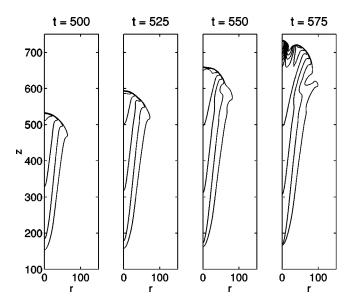
FIG. 1. Evolution of an anode directed streamer in a strong homogeneous background field. The planar cathode is located at z=0 and the planar anode at z=2000. The radial coordinate extends from the origin up to r=2000 to assure homogeneous field conditions. Shown is  $100 \le z \le 750$  and  $0 \le r \le 150$  with equal axis scaling. The thin lines denote levels of equal electron density  $\sigma$  with increments of 0.15. All plotted quantities are dimensionless.
