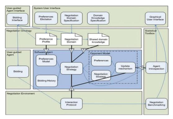
FIGURE 2. GENIUS's detailed architecture.
