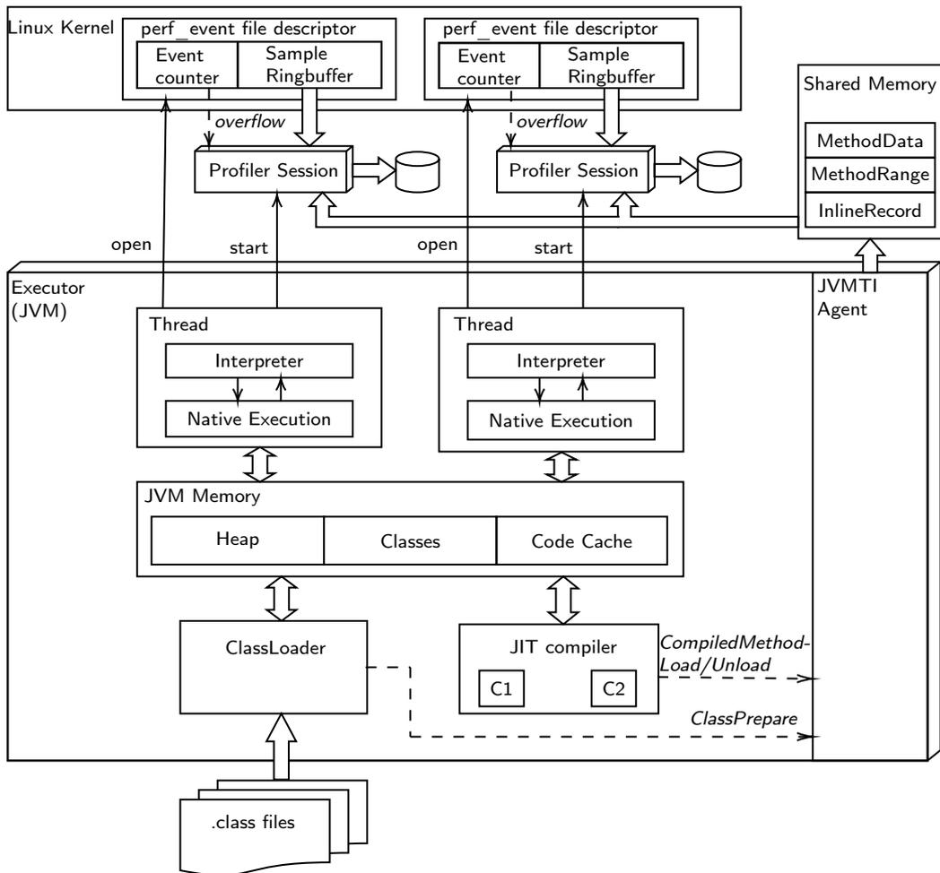
Figure 4.1: Overview of the LLSS profiler design.
