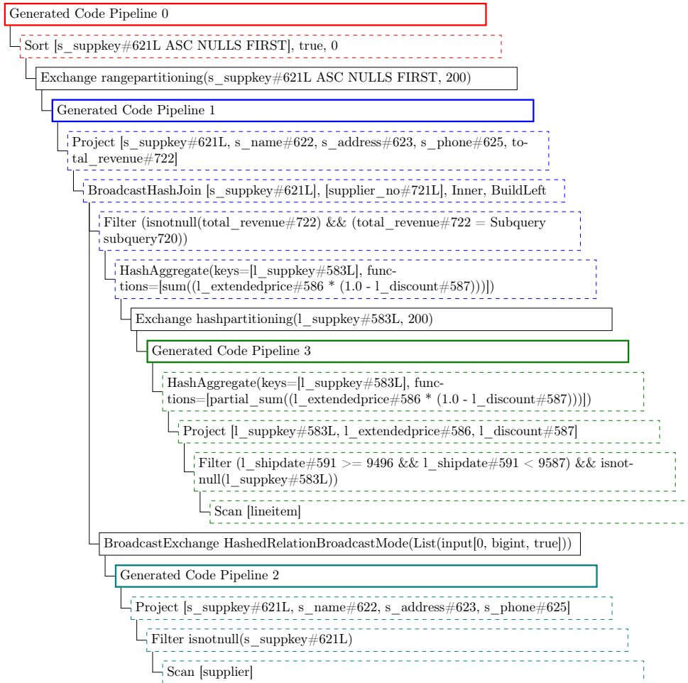
Figure 2.2: The physical plan for query Q15 in the TPC-H benchmark, illustrating the common occurrence of the operators project , broadcast hash join , filter , hash aggregate and scan in the compiled pipelines of an optimized SQL query.
