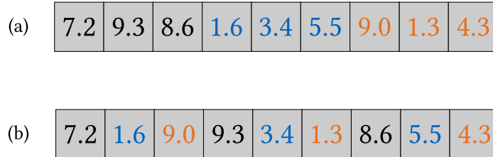
Figure 2.1: Storage of 3 embeddings in the (a) horizontal and (b) vertical layout
