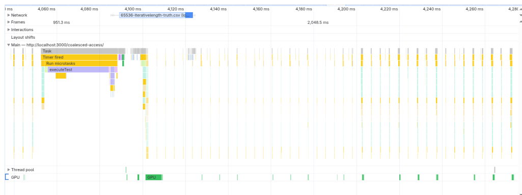
Figure 5.13: Shows the profiler trace for one run of the IBFS algorithm. Note that there are long pauses between any GPU work being executed. These pauses are there due to the added overhead of communication between WebGPU and the CPU, resulting from the browser’s event loop.
