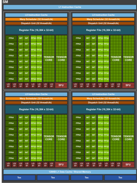
(a) GPU SM architecture as described for the Tesla V100 (NVIDIA). Each SM contains four execution units, which share L1 Cache and texture units. Each execution unit has its own ALUs, scheduler, register file, instruction cache and dispatch unit.
