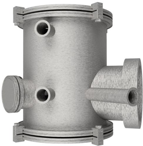
**Figure A1.** The geometry of the experimental discharge vessel, as seen from the side. It is a quasi-cylindrical vessel that contains observation windows and gas flow tubes. The ICCD camera captures pictures through large window on the right. We observed that streamers propagated slightly off-axis, with the deviation toward the largest window, which is most likely related to the electric potential distribution inside the vessel, see section 4.9.
