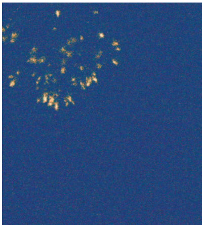
Figure 1: Two views of a streamer (the phase immediately preceding a discharge). To the left a time integrated picture (exposure time 10^{-6} seconds); to the right a snapshot of the same event (exposure time 10^{-9} seconds), showing the propagating heads of the streamer channels. (Courtesy E. van Veldhuizen, Eindhoven University of Technology.)
