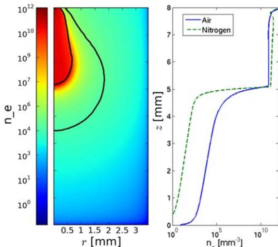
Fig. 3. left: Electron density in  $\text{mm}^{-3}$  of a positive streamer in air. Black line indicates where the electric field exceeds the breakdown value. Right: Electron densities on the axis of positive streamers in air (solid line) and  $\text{N}_2$  with a 1 ppm  $\text{O}_2$  admixture (dashed line).
