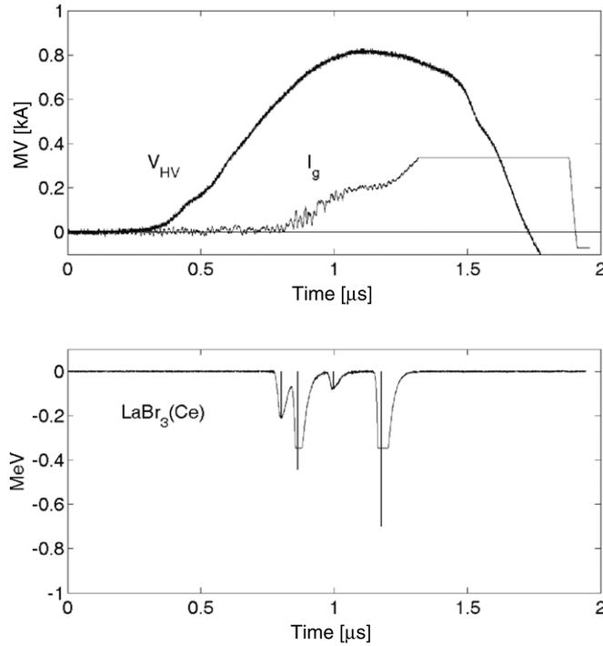
**Figure 4.** Positive surge with 810 kV maximum, shown with the current  $I_g$  during the leader initiation phase. At  $1.5 \mu\text{s}$  the gap breaks down. Four x-ray pulses can be distinguished. The  $\gamma$ -detector and current signals are clipped by the oscilloscope. The vertical bars indicate the maximum equivalent energy and its timing obtained by the fit.
