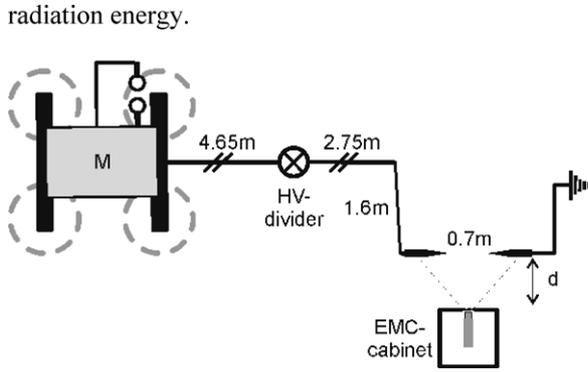
**Figure 1.** Floor plan of the setup, showing the position of Marx generator (M), HV divider, 0.7 m spark gap and EMC cabinet with detector at the distance  $d$  from the gap.
