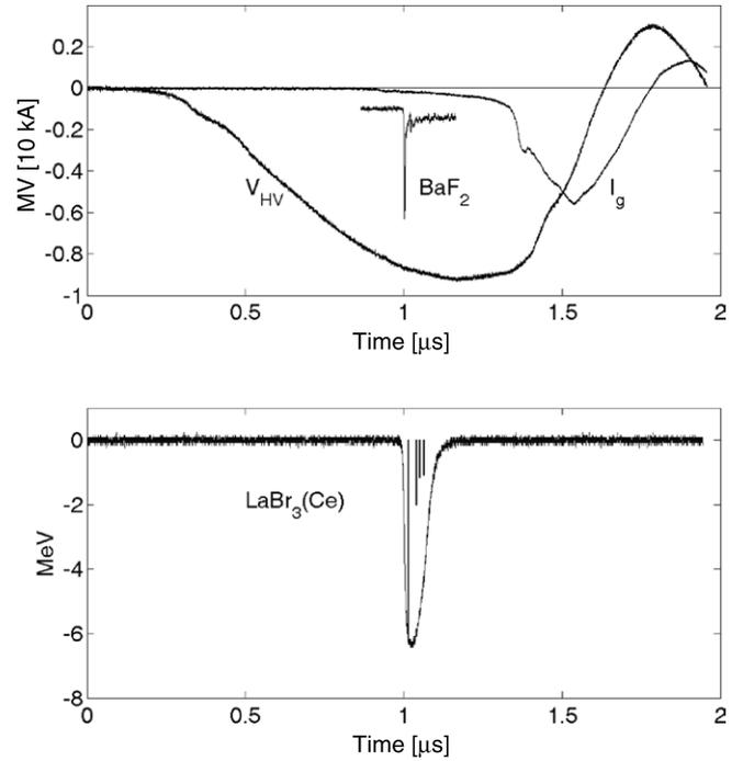
**Figure 5.** A negative 875 kV surge, shown with the current  $I_g$  and x-ray signal (arbitrary units) from an uncalibrated  $\text{BaF}_2$  detector alongside the  $\text{LaBr}_3(\text{Ce})$  detector. The lower part of the figure shows the signal of the  $\text{LaBr}_3(\text{Ce})$  detector and the fitted amplitudes of a train of four pulses.
