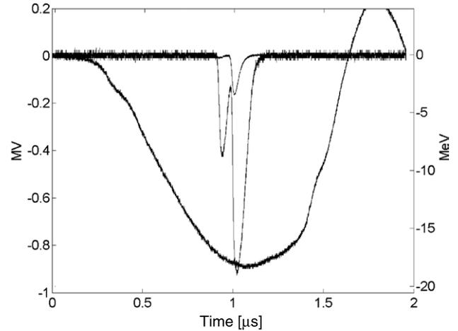
**Figure 7.** Negative surge (left ordinate) and x-ray signals (right ordinate) seen by two detectors, one without (large signal) and one with (smaller signal) a 1.5 mm Pb absorber.
