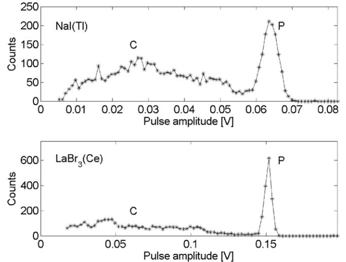
**Figure 2.**  $^{137}\text{Cs}$  pulse height spectrum for NaI(Tl) and LaBr<sub>3</sub>(Ce) detectors of 5000 pulses recorded by an 8 bit resolution oscilloscope. The horizontal axes have been scaled to coincide on the photopeak.
