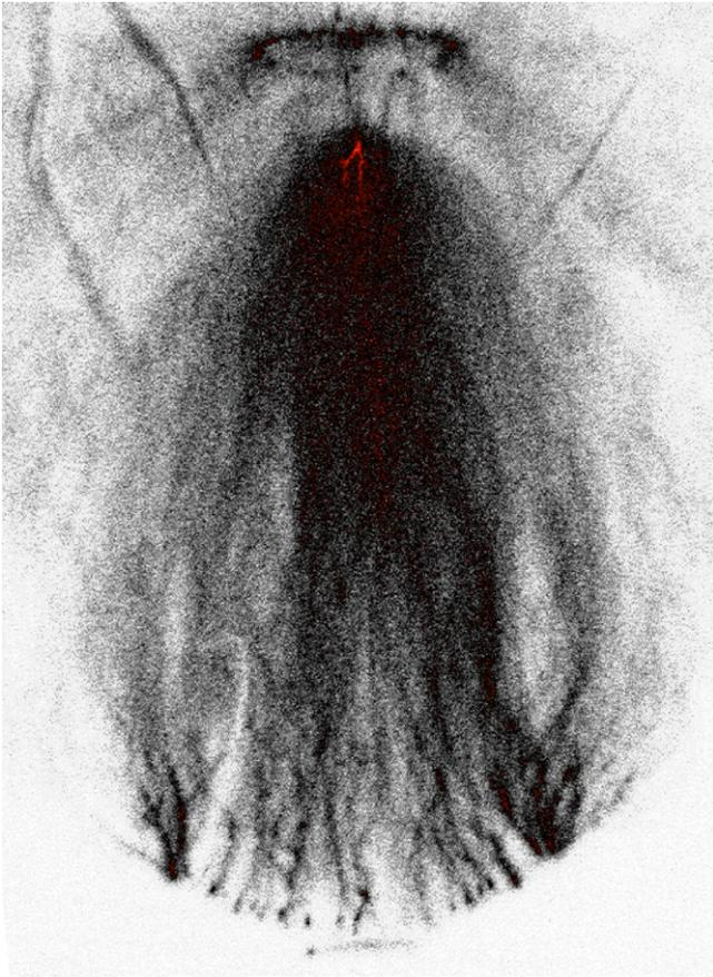
**Figure 7.** Connection between positive downward and negative upward streamers initiated from the sharp belt. Exposure time is 300 ns; the gap length is 1 m.
