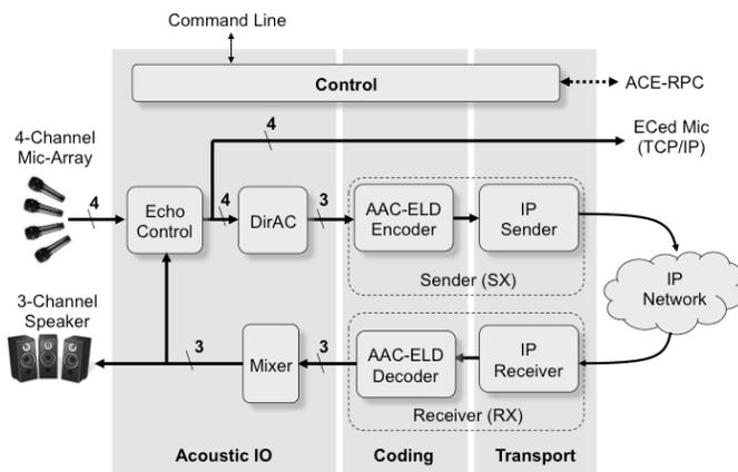
**Figure 8: Components of the Audio Communication Engine (ACE).**
