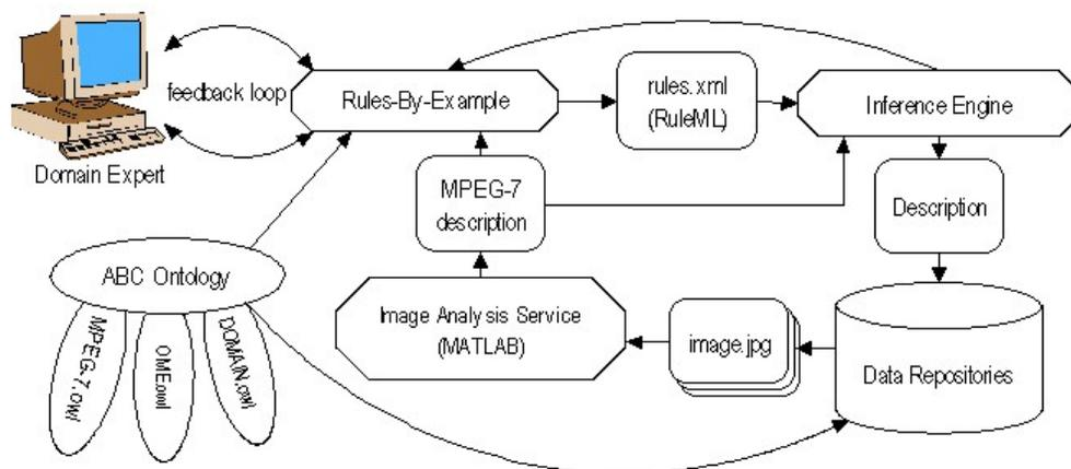
**Figure 3.4** Architecture for the RBE System.
