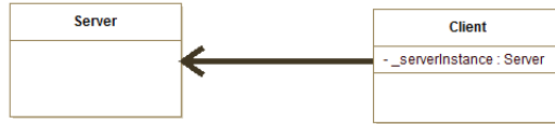
Figure 2.1: Example of a client class being coupled to the server class by a private field.
