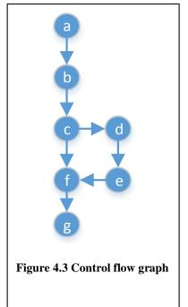
To illustrate the conversion from a method to a control flow graph, consider the method shown in figure 4.2. The statements which use the SharePoint API are underlined. All the other statements are disregarded during tracing. Figure 4.3 shows the control flow graph after the method is traced. Two execution paths can be identified  $\{a,b,c,f,g\}$  and  $\{a,b,c,d,e,f,g\}$  which translate into:
