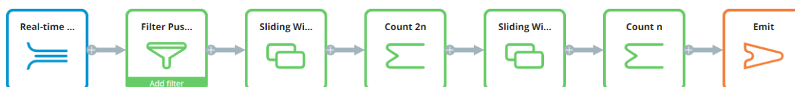
Figure 8.2: GitHub PushEvent flattened trend strategy. Semantically this is the same as the figure above, but the intent of this strategy is arguably harder to understand without splitting the stream.
