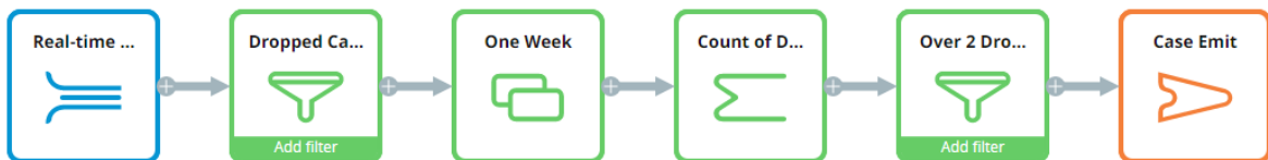
Figure 3.1: Example event strategy: the first shape is the source and emits events as they arrive in real time; the second shape is a filter that selects dropped call events; the next two shapes combine a sliding window of one week with a count aggregate; the fifth shape is a filter that selects the third (or more) dropped call; the last shape is the emit, in this case the emit strategy only emits the first event within the window and triggers an action.
