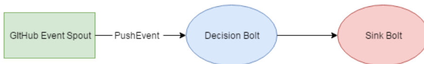
Figure 9.2: Storm topology for the push event trending scenario where the knowledge of the event filter is pulled up to the spout. Only events of the type PushEvent are transferred to the decisioning bolt.
