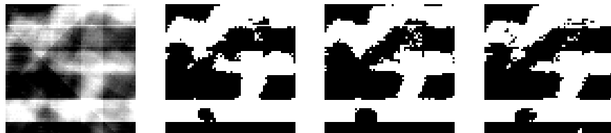
Fig. 4. (a) ART reconstruction of the image in Fig. 3b from 6 projections; (b) Rounded ART reconstruction; (c) Solution of Problem 2, using the ART reconstruction as the weight map, for lattice directions (1, 0) and (0, 1) ; (d) Solution of Problem 2 using lattice directions (0, 1) and (1, 1) .
