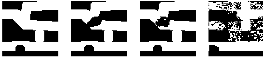
Fig. 3. (a) Blueprint image of a semiconductor part; (b) Test image, containing a gap in one of the wires; (c) Reconstruction of the test image from the horizontal and vertical projections, using the image from (a) as a model image; (d) Reconstruction using an inverted version of the blueprint image as a model image.
