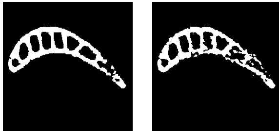
Figure 12: (a) (Left) R-FIB reconstruction from 6 projections. (b) (Right) Network flow reconstruction from 6 projections.
