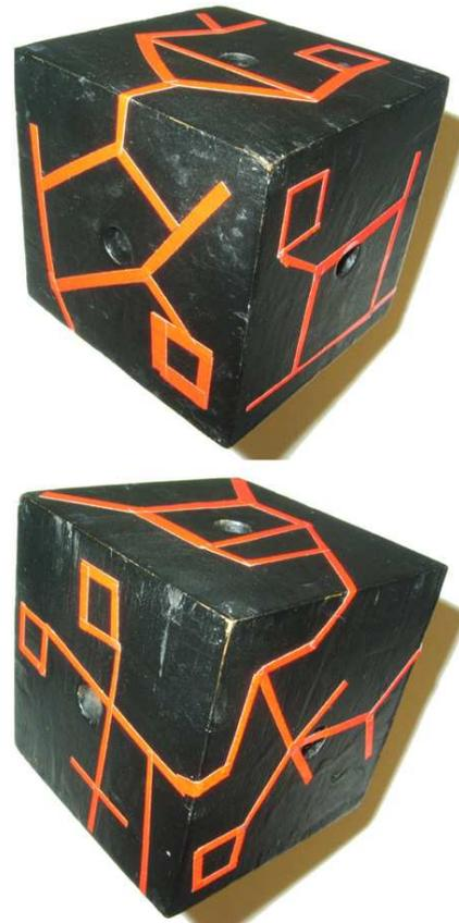
Fig. 1. A  $7 \times 7 \times 7$  cm cubical input device augmented by a graph pattern of retro-reflective markers. All six faces of the cube are shown. Note that graph edges are allowed to cross over between faces of the cube and do not need to be straight lines.
