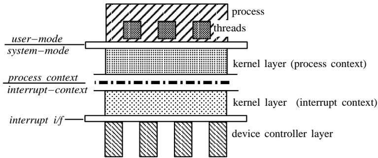
**Figure 3:** Elements of the UNIX processing hierarchy.
