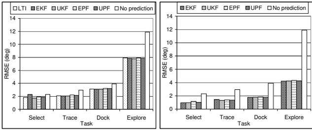
Figure 7: Filter comparison for  $t_{pred} = 66$  ms,  $f_s = 60$  Hz,  $N_z$  10 and 3 times the nominal orientation and angular velocity measurement noise, respectively, using (a) only orientation measurements (MM), and (b) including inertial measurements (MMI).
