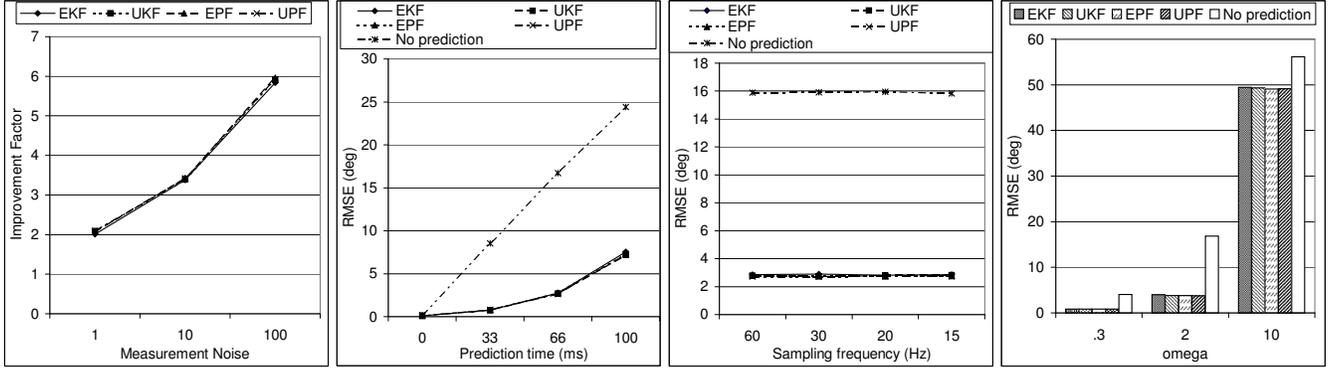
Figure 4: Synthetic results: (a) Improvement factor vs. measurement noise ( $\omega = 2$ ). (b) RMSE vs. prediction time ( $\omega = 2$ ). (c) RMSE vs. sampling frequency ( $\omega = 0.3$ ). (d) Filter comparison for  $t_{pred} = 66$  ms,  $f_s = 60$  Hz,  $N_z = 10$  and 3 times the nominal orientation and angular velocity measurement noise
