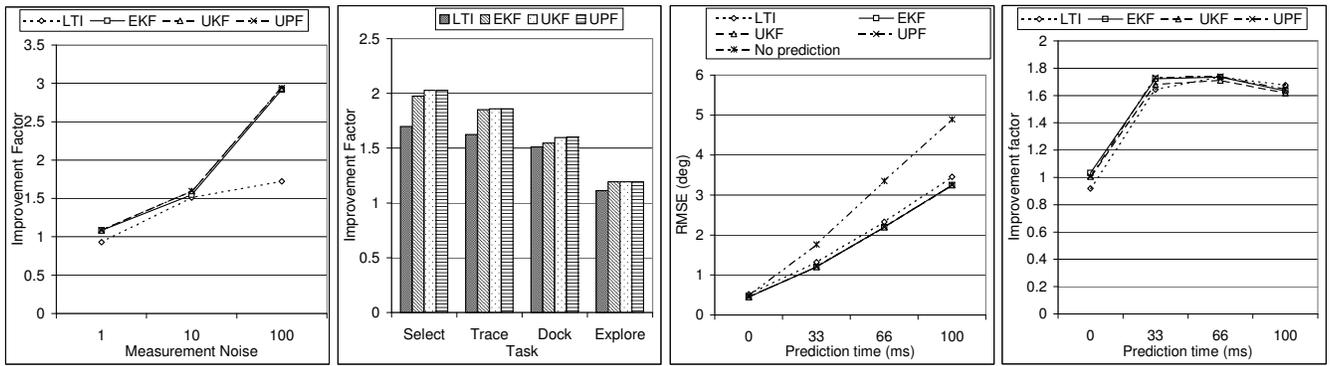
Figure 5: Filter results: (a) Improvement factor vs. measurement noise (docking task). (b) Improvement factor vs. task for 10 times  $N_z$ . Prediction results: (c) RMSE vs. prediction time (docking task). (d) Improvement factor vs. prediction time (exploration task)
