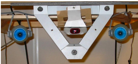
Figure 5: The two iBOT cameras mounted in a PSS prototype next to the Logitech emitter.
