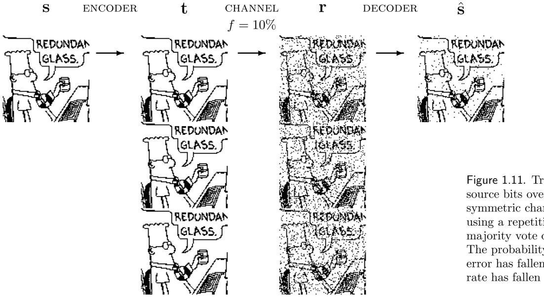
Figure 1.11. Transmitting 10000 source bits over a binary symmetric channel with f = 10%using a repetition code and the majority vote decoding algorithm. The probability of decoded bit error has fallen to about 3%; the rate has fallen to 1/3.
